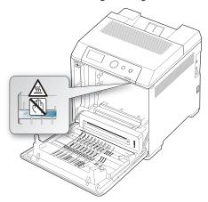
When you open the front cover and work inside the machine, it is highly recommend that you remove the paper transfer belt first. Because the work you do could contaminate the paper transfer belt.
